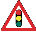
Traffic Signals Ahead
