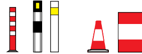
Delineators (used to mark the edge of the road or traffic island)
