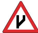
Start of Dual Roadway (Straight On)
