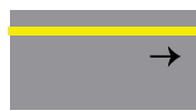
Left Edge Line On one way roads the right edge line is white
